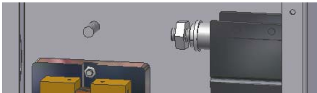
5/16" stud for battery negative tie point
